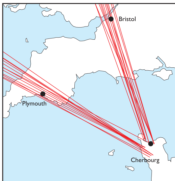
Figure 5.5: The threat of V1 missiles to the South West. The lines of flight were projected from aerial photographs showing the orientation of the launch ramps on the Cherbourg peninsula. The missiles could be timed to fall onto targets along the line (after Babington Smith 1957).
