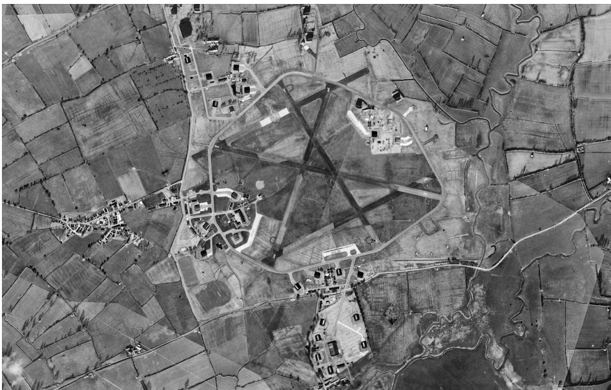
Figure 2.12: Post-war aerial photograph of RNAS Henstridge on the Somerset/Dorset border, showing the five-runway layout with outlying accommodation and technical areas. The dummy carrier deck can clearly be seen on the most northerly runway (Somerset Studies Library, RAF CPE/UK/1974 4170, 11/4/1947).
