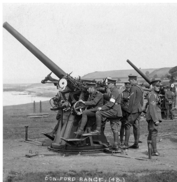
Figure 4.7: A 3-inch anti-aircraft gun on the Doniford ranges before the war. The same type was used at Uphill in both anti-aircraft and anti-shipping roles (courtesy Vernon Stone from a postcard by HH Hole).
