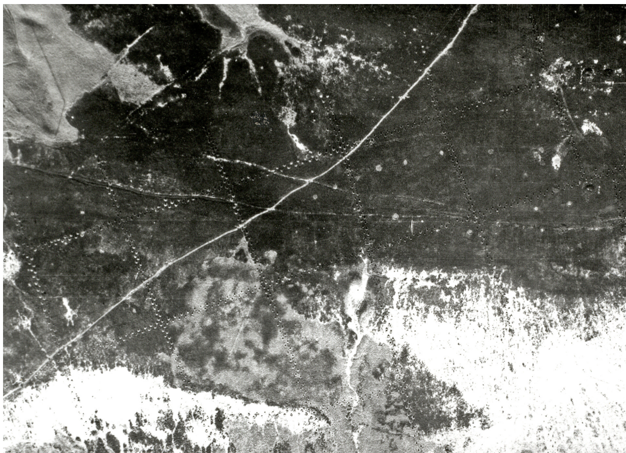
Figure 3.4: Aircraft landing obstructions on the open moorland of Black Down near Shipham. These obstructions were constructed of double lines of heaps of stone or turf. It is likely that they survived wartime clearance for agriculture because the site was used for several bombing decoys (Somerset Studies Library, RAF 3G/TUD/UK/15/25/PART I 5279, 14/1/1946).
