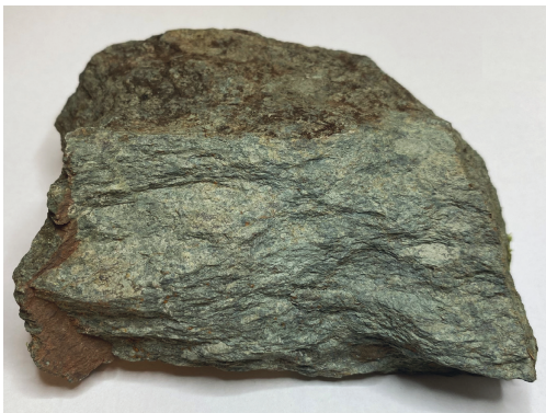
Fig. 3 Hand specimen of Cockercombe Tuff collected from Dibbles Quarry in February 2023 showing the characteristic grey-green colouration and silvery sheen on fresh faces (sample length 115mm). (Image and all following): Andy King
