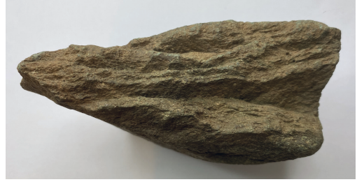
Fig. 4 Side view of a hand specimen of brown weathered Cockercombe Tuff collected from Dibbles Quarry in February 2023 showing cross-bedding and coarse lamination indicating deposition under water (sample length 125mm).
