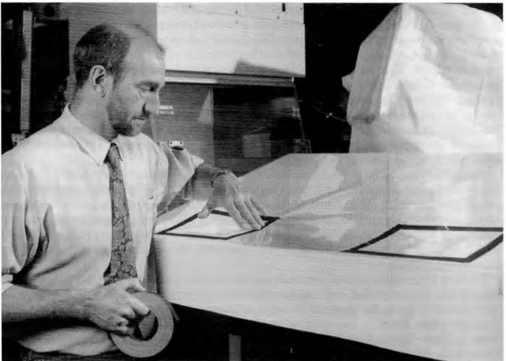
Fig. 2 Dennis Parsons constructing the dust box within which the specimen was prepared
