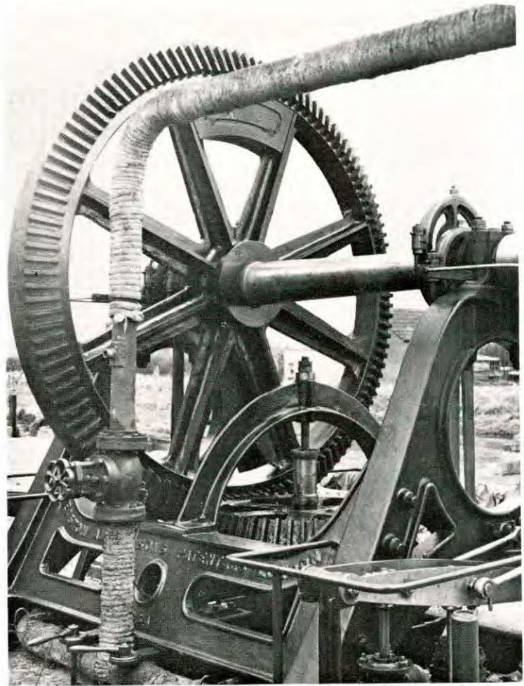
PL. IB Curry Moor Steam Pumping Engine, built by Easton, Amos and Sons in 1864. Though no longer in use it remains at its original site protected from the weather by a new house. The site can be seen in Pl. IA.
