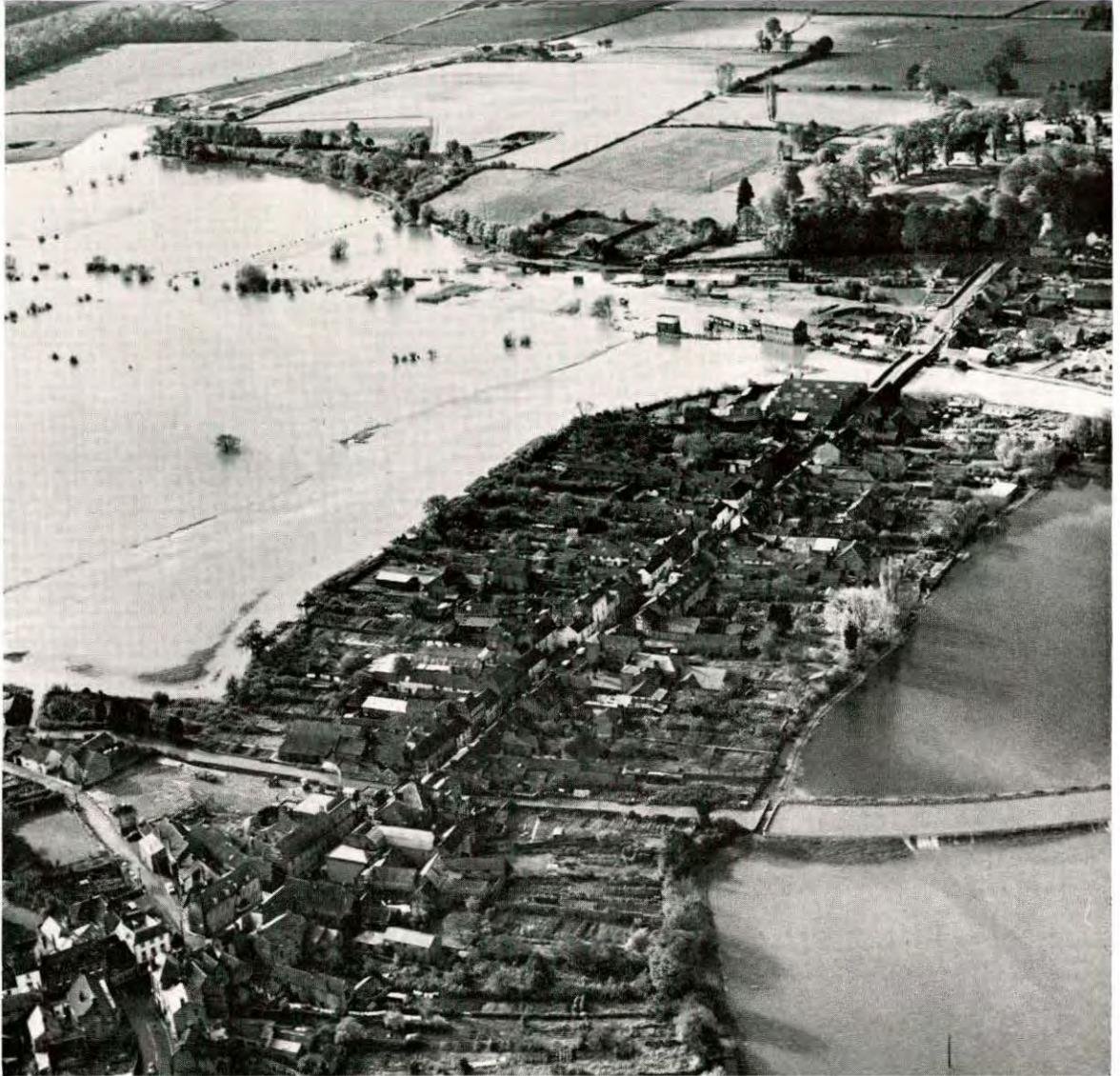
PL. III Langport, showing the bottleneck at Great Bow Bridge (top right), through which the drainage of about 190,000 acres must flow. The channel flowing across the lower half of the picture is the Long Sutton Catchwater, which is no longer used and much of which has been filled in.
