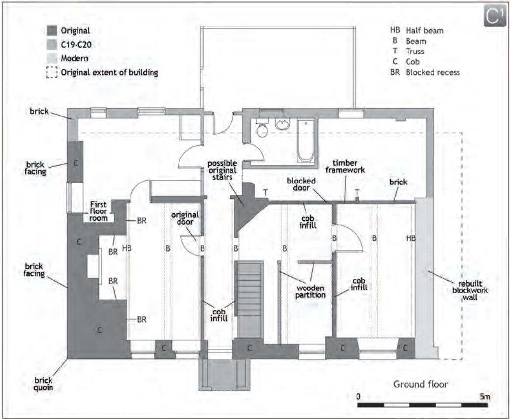
Fig. 5 Schematic reconstruction – phased ground floor plan
