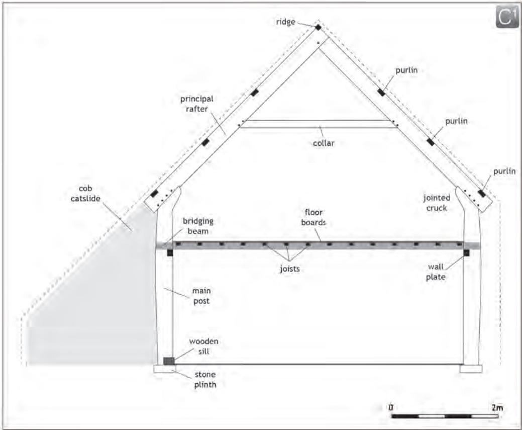
*Fig. 2 Schematic reconstruction - cross-section*
