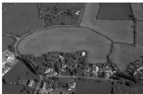
Fig. 4 Aerial view of the oval shaped 'summer dike' (Church Field) at Puxton. These small enclosures were built around the 10th century on the surface of a high saltmarsh in order to prevent summer flooding of cultivated areas
