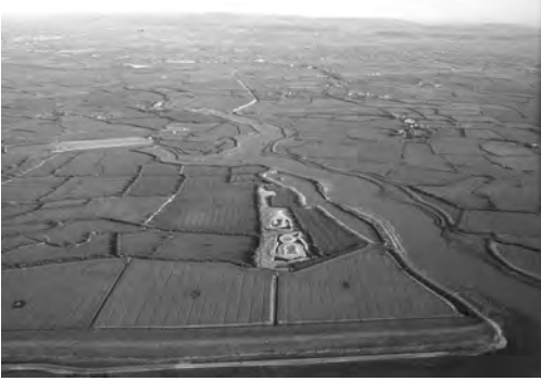
Fig. 5 Aerial view of the estuary of the Congresbury Yeo, showing the sea walls constructed to completely protect the North Somerset Levels from tidal inundation. The historic landscape was then created behind them through the gradual process of enclosure and drainage, as population and the demand for agricultural land increased throughout the medieval and post-medieval periods
