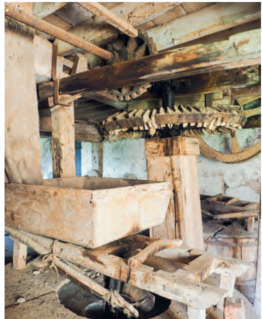
Fig. 4 Milverton Mill, Crown wheel with drive to two pairs of grinding stones and threshing wheel
