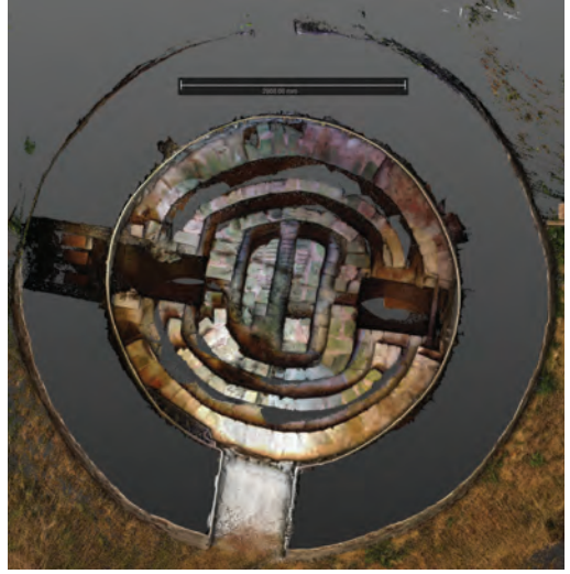
Fig. 4 Plan of the fireboxes and labyrinth of flues beneath the original floor (north at the top). Note the meltdown of the brickwork of the westernmost flue.
