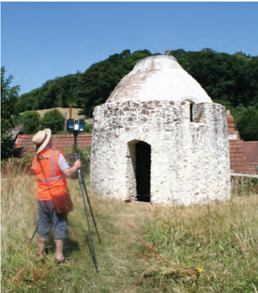
Fig. 1 Bill Stebbing surveying the kiln using a Faro Focus laser scanner
