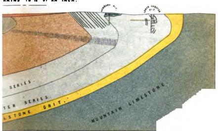
or slide fault, which was discovered many years ago in working the Radstock series of veins.
